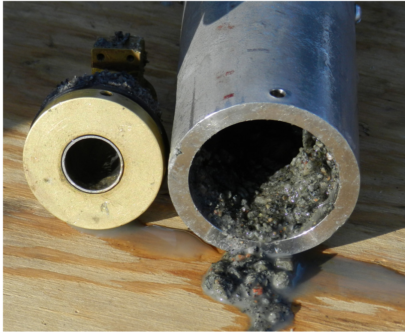
Figure 3-7. Photograph showing sample of bed material collected in a 700 m ice borehole GL 12-2B located about 30 km from the terminus. Sand size grains dominate the sample and fine grains and clays are notably lacking.
