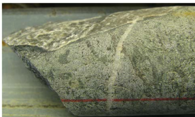
Figure 5-79. Synchronous, practically mono-mineral gypsum fracture infillings sealing two fractures with different orientations (DH-GAP04, 533 m). The cross-fibrous texture is very common and indicates mineral growth during extensional conditions. Photograph by Tuomas Pere.
