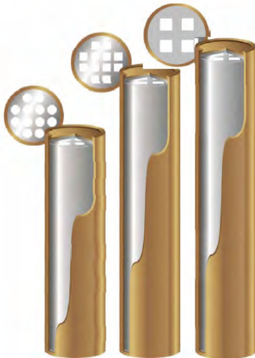
Figure 6-5. Copper-iron canisters for the spent nuclear fuel from the LO1–2 , OL1–2 and OL3 reactors from left to right (Raiko 2005). All versions of the canister have the same outer diameter of 1.05 m. The height ranges from 3.6 to 5.2 m.
