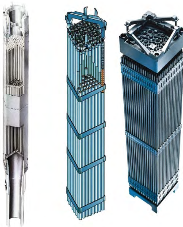
Figure 6-4. Representative illustrations (from left) VVER-440 (LO1-2), BWR (OL1-2) and OL3 type fuel assemblies. BWR and VVER-440 fuel elements are partly cut open to show the internal structures. The pictures are not to scale.
