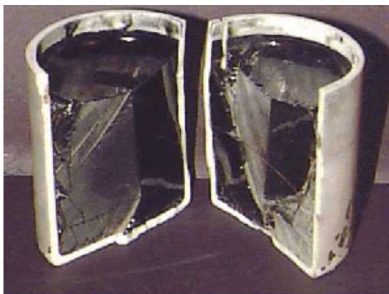
Figure 2.1.1-1. Section through a steel canister containing vitrified HLW ( http://nuclearstreet.com/images/img/dw117.jpg )
