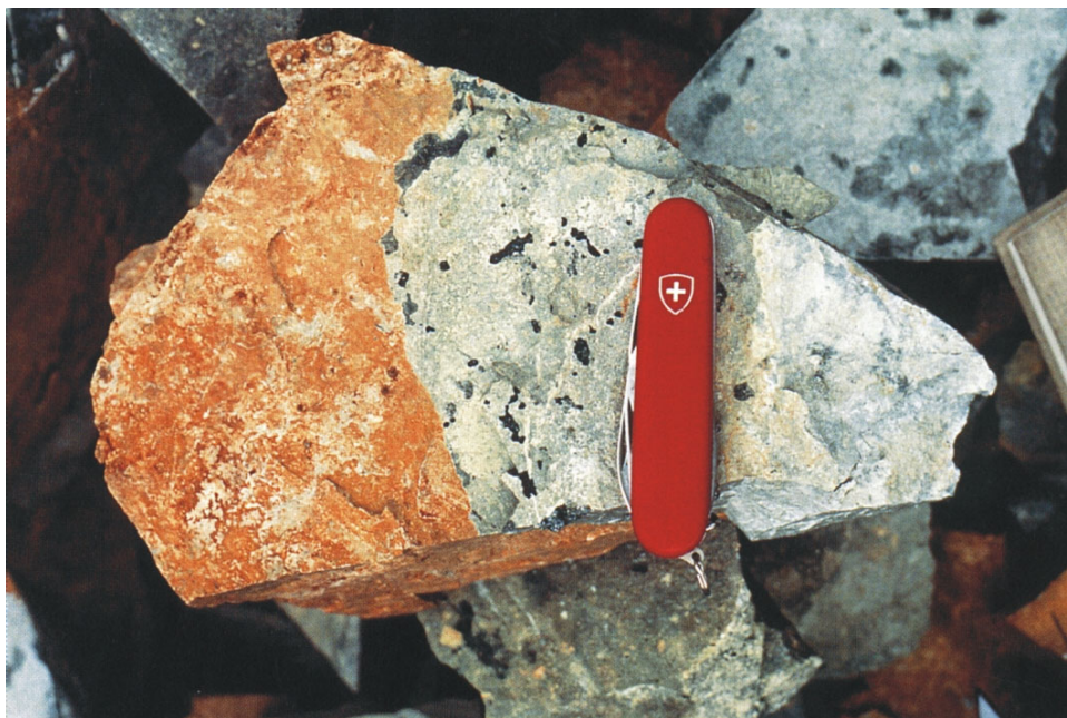
Figure 8.2-2. A hand specimen from the Osamu Utsumi mine showing the redox front, formed by the percolation of oxygenated surface water into the rock. Unoxidised rock is blue-grey, right, oxidised rock is red-brown, left. (Miller et al. 2000)
