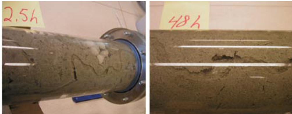
Figure 9.3: Photographs of bentonite pellets in a Plexiglas tube being filled with water (left) and of channels later formed by piping (left and right) (Figure A16.4 of R-06-72, Börgesson and Sandén 2008).
