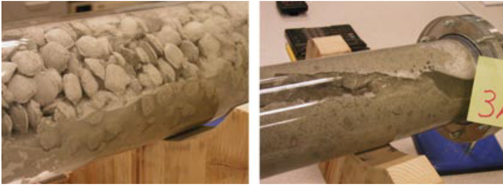
Figure 9.2: Photographs of bentonite pellets in a Plexiglas tube being filled with water (left) and of a channel later formed by piping (right) (Figure A14.4 of R-06-72, Börgesson and Sandén 2008).
