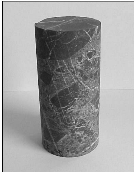
Figure 5. A typical sample gained from a Cretaceous tectonic zone, as an evidence of paleo-self-healing
