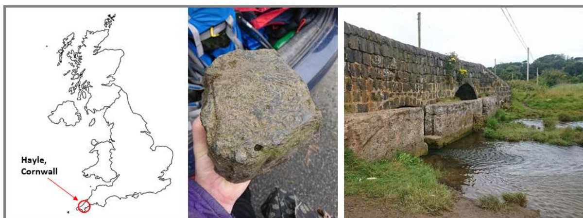
Figure 7: Left , location of Hayle, Cornwall, UK, middle , a vitreous slag sample, right , slag sample held in position for 250 years by inclusion in a bridge across the Hayle estuary.
