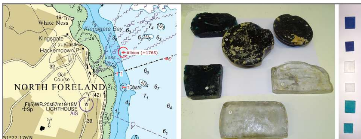
Figure 6: Left , location of the shipwreck of the Albion where the glass ingots were found, middle and right , images of the ingots coloured blue (Co), clear (Mn) and green (Cu).
