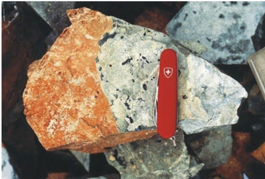
Figure 7.2-2. Small-scale redox front in a rock sample (note knife for scale). The orange-red area on the left is the oxidising zone, the grey area on the right is the reducing zone (Waber et al. 1990).
