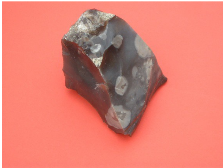
Figure 2.1.1-2. Obsidian from the Ross of Mull, Scotland (Anderson and Radley, 1915). Note the grey-white spherical zones of devitrification within the otherwise glassy matrix in this approximately 60 million year old glass (H.A.Alexander, Bedrock Geosciences, Switzerland).
