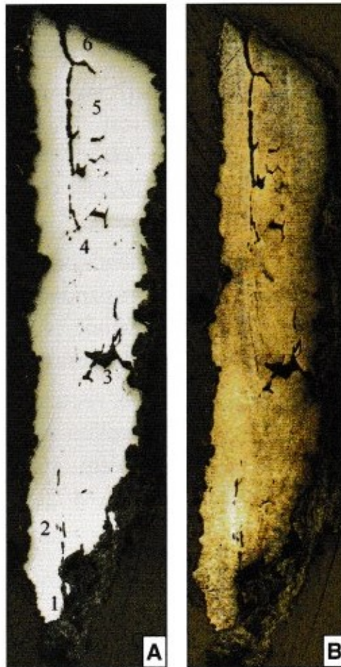
Figure 3.2-2. An unidentified steel artefact from the Broxmouth hillfort. Approximately 2 cm long, it is made from high carbon steel which has been heat-treated and quenched. A etched, B unetched (Armit & McKenzie 2013).
