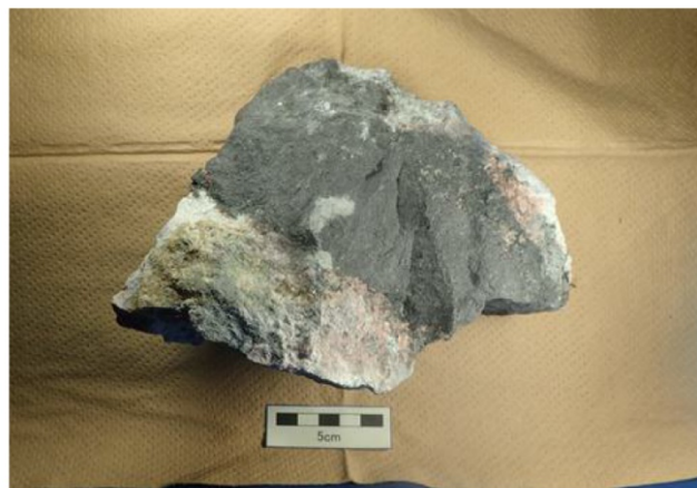
Figure 5.1.8-2. Sample collected in the Kiruna mine for Work Package 5 analysis (sample 1-1). Dark material (upper half of the sample) is the ore (predominantly magnetite) and the lighter material (bottom half of the sample) the bentonite (Sato et al. 2021).
