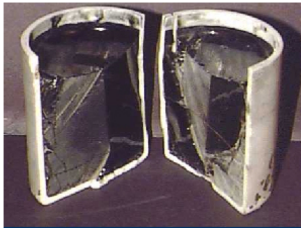
Figure 2.1.1-1. Section through a steel canister containing vitrified HLW ( http://nuclearstreet.com/images/img/dw117.jpg )
