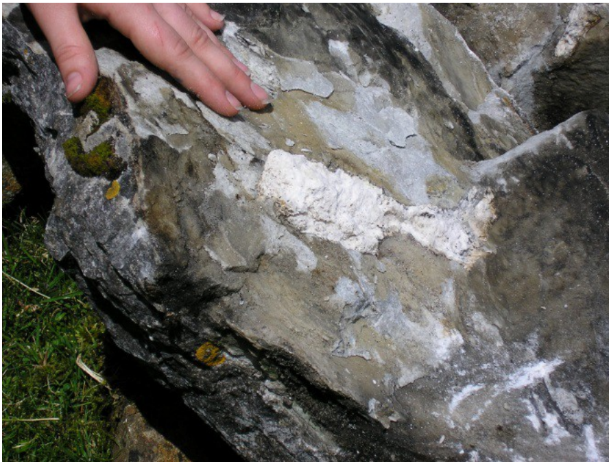
Figure 4.1.4-2. Hydrous gel-like phase formed by hydration and alteration of a larnite nodule, which was revealed in a freshly broken block of rock from Scawt Hill (Milodowski et al. 2011).
