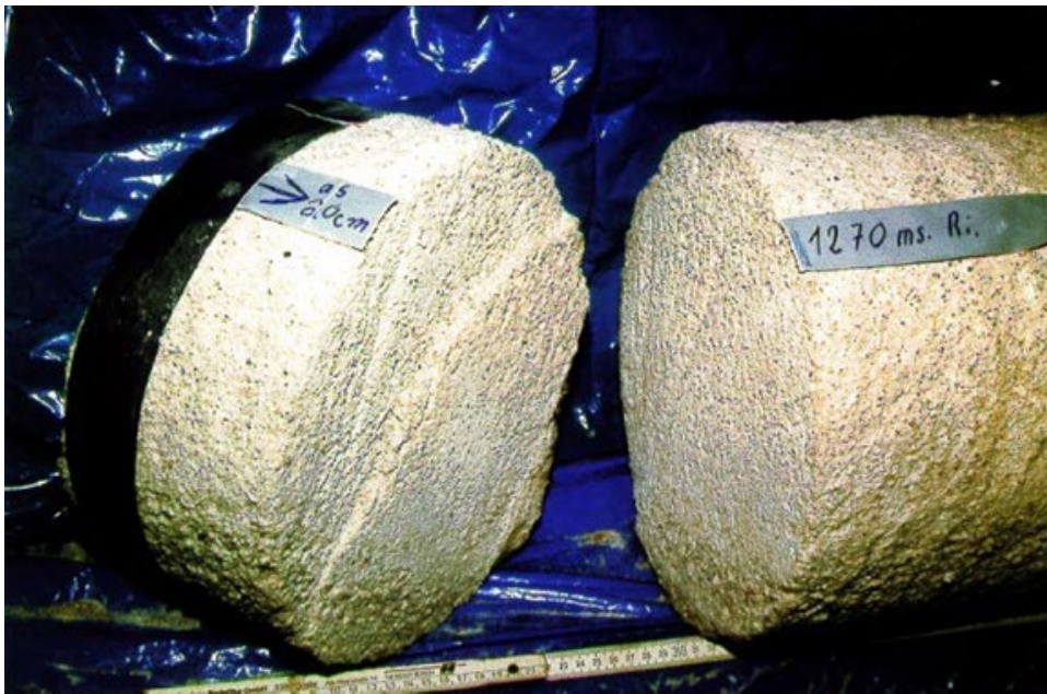
Figure 6.4.2-1. Core through 20 year old compacted salt (from the Riedel mine, Germany), taken to assess void reduction efficiency with time. (Brenner et al. 1999).
