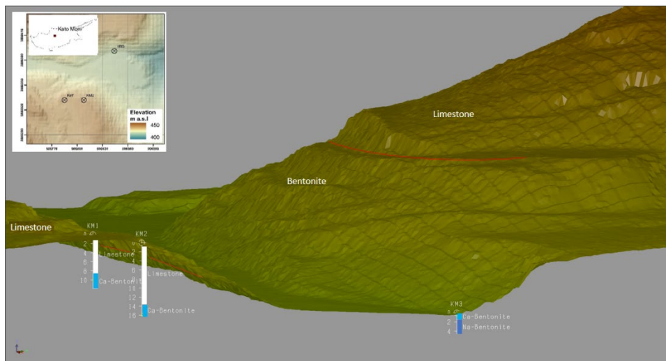
Figure 5.1.3-3. 3D model of the Kato Moni (Cyprus) quarry topography (view looking to the NW). Boreholes KM1-KM3 (depths shown in meters) with KM1 and KM2 drilled through limestone (white) into the bentonite (blue) beneath and KM3 drilled straight into bentonite (blue colours). Red line shows the bentonite - limestone boundary at the northern and southern hill slopes (modified from Reijonen et al. 2017).
