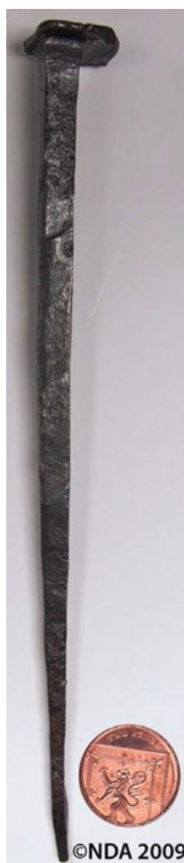
Figure 3.2.1-3. An example of a remarkably preserved nail from the Roman hoard at Inchtuthil, Scotland (NDA).
