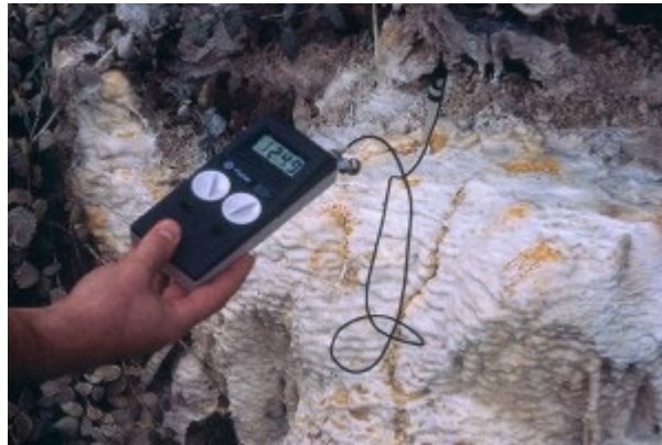
Figure 3-22. Image from SKB's Swedish-language web site showing high pH natural groundwaters at the Maqarin site in northern Jordan as part of a discussion on the reaction of cement leachates with a GDF host rock.
