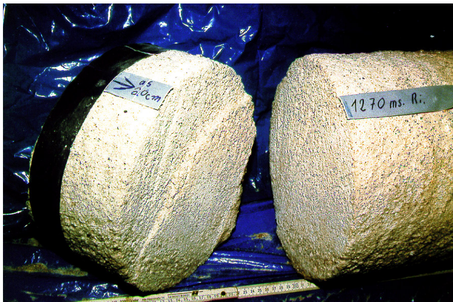
Figure 1: Final segments of a core drilled into old backfill from the 1260/1275 m floor of Riedel salt mine.
