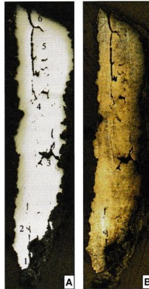
Figure 4: an example of the steel artefacts identified at the Broxmouth Hillfort site (A unetched, B etched). Sample is 19.5 x 5.5 mm [10]
