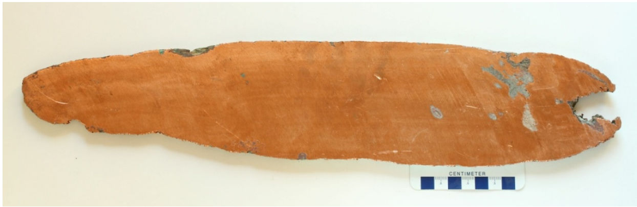
Figure 2. Cut slab from a mass of float copper from Quaternary deposit showing a thin layer of surface alteration on surface and silicate inclusions.
