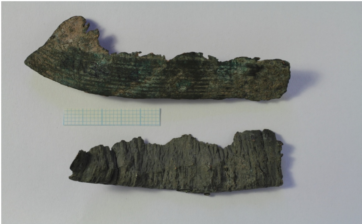
Figure 3. Chisel chips carved by miners showing surface oxidation after exposure for approximately 150 years.
