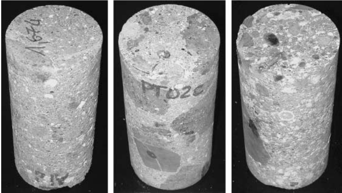
Figure 3: Typical low alkali cement core samples recovered from archaeological sites at Portus and Anzio, Italy [12]
