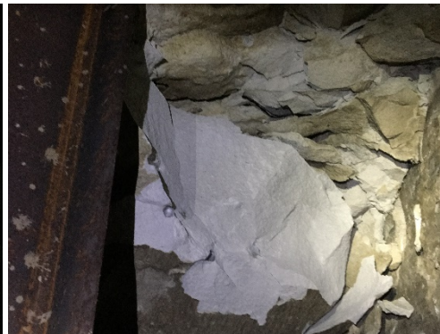
Bentonite rock samples collected from the tunnel wall
