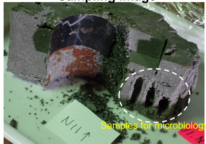
Sampling positions in the bentonite buffer material
